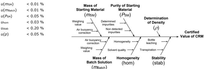
The combined standard uncertainty is calculated by combination of the standard uncertainties of the input estimates according to Eurachem/CITAC Guide "Quantifying Uncertainty in Analytical Measurement" and ISO 17034. [2][4]
