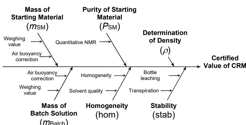
The combined standard uncertainty is calculated by combination of the standard uncertainties of the input estimates according to Eurachem/CITAC Guide "Quantifying Uncertainty in Analytical Measurement" and ISO 17034. [2][5]
