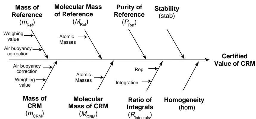
The combined standard uncertainty is calculated by combination of the standard uncertainties of the input estimates according to Eurachem/CITAC Guide "Quantifying Uncertainty in Analytical Measurement" and ISO 17034.<sup>[2][5]</sup>
