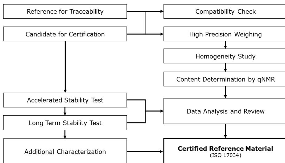
**Homogeneity assessment:** Homogeneity of the material is tested by qNMR measurements using 5-10 subsamples which are taken from different positions in the entire bulk material. The recommended minimal sample size is taken for all the homogeneity test samples. Analysis of variance (ANOVA) results are included into the calculation of content uncertainty of this CRM.
