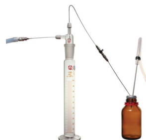
Fig. 12 Double-tipped needle transfer to graduated cylinder
