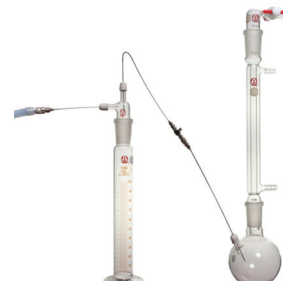
Fig. 13 Double-ended needle transfer with syringe valve
