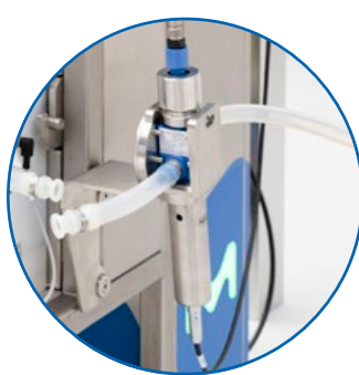
Pre-column instrumentation for conductivity and pH measurement
