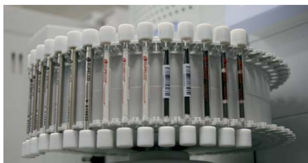
A Variety of Supelco Thermal Desorption Tubes in Autosampler
