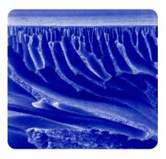
**Figure 2.** Conventional 10 kD polyethersulfone membrane with sub-surface voids
