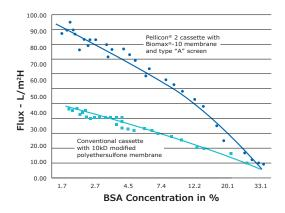
Figure 3. Flux versus BSA concentration
