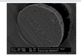
**Figure 2b**. SEM Image of the Interior of a Pd(OAc)<sub>2</sub>-Containing Microcapsule. (Photo courtesy of Avecia Ltd, and is reproduced with permission.)
