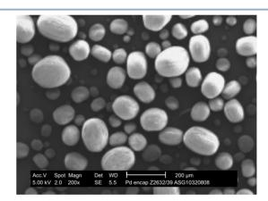
Figure 2a. Scanning Electron Microscope (SEM) Image of Microcapsules Containing Pd(OAc)<sub>2</sub>.
