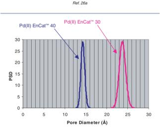
Figure 3. Pore Size Distribution (PSD) for Pd(II) EnCat<sup>™</sup> 30 and Pd(II) EnCat<sup>™</sup> 40 in the Tetrahydrofuran-Swollen State as Determined by Chromatographic Porosimetry. (Graph courtesy of Avecia Ltd, and is reproduced with permission.)
