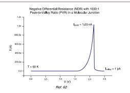
**Figure 3.** Current as a Function of Voltage [I(V)] Characteristics of a Nanopore Test Bed Device Containing a SAM of Molecule **58** at 60 K. The Peak Current Density Is ~50 A/cm<sup>2</sup>, and the Peak-to-Valley Ratio (PVR) of the Negative Differential Resistance (NDR) Response is 1030:1.
