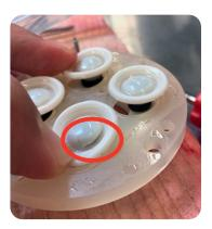
Figure 12. Pump chamber diaphragm failure.
