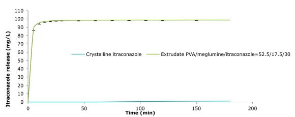
Figure 2: Dissolution of itraconazole (900 mL SGF, 37 °C, 100 rpm, 100 mg itraconazole, 30 % drug load; N=3).
