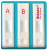
Hbs Ag antigen detection assay used as model lateral flow test. Estapor® K1-040 Red Intense shows superior sensitivity compared to competitor A and B even at low conjugation concentration.
