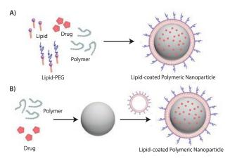
Figure 1. Schematic showing one- and two-step LPN synthesis. A) One-step synthesis method. B) Two-step synthesis method.
