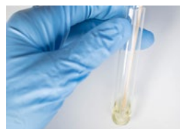
Transfer swab into 2 mL dilution broth (Lethen Broth) and vortex
