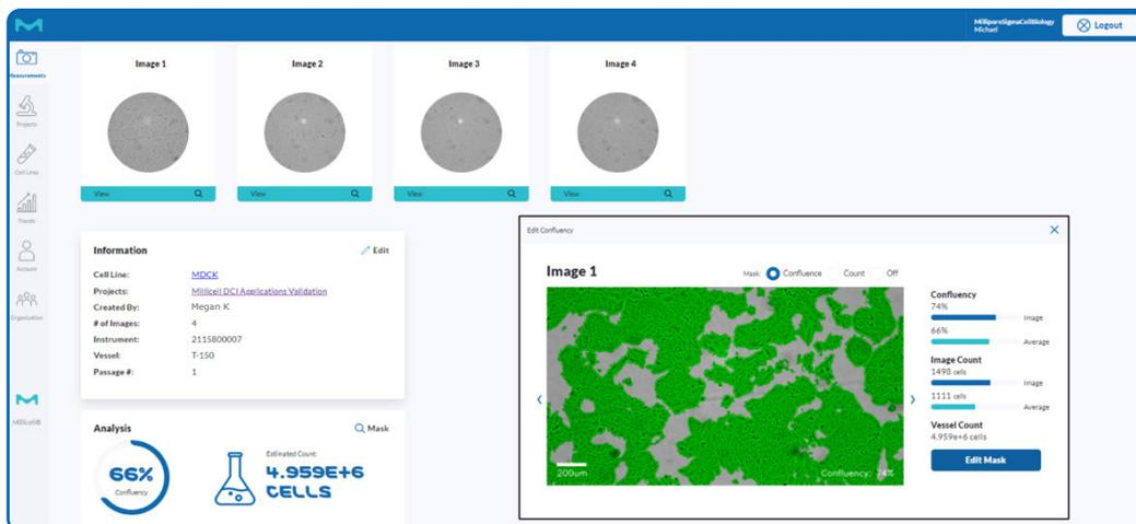
A culture of MDCK cells was measured directly in a T-150 flask using the Millicell® DCI. From Image 1, confluency was determined to be 74% with 1,498 cells in the field of view. Using the average of four separate images, the culture was determined to be 66% confluent with an estimated total cell count of  $4.959 \times 10^6$  cells.
