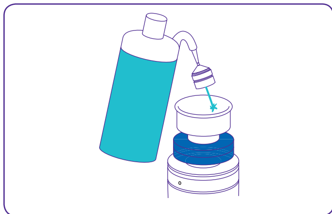
Figure 30. Wash down inside of funnel.
