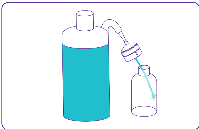
Figure 33. Rinse inside of sample collection container.
