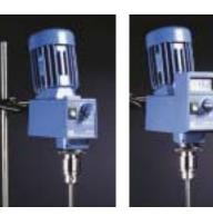
Two speed ranges for stirring applications up to 20L (in terms of H<sub>2</sub>O) of material. 292 H x 88 W x 188mm D. Wt = 2.9kg. Order stirring shafts separately; see listings in the Aldrich Handbook. CE compliant.
