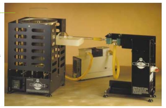
Kugelrohr apparatus shown with KNF Laboport vacuum pump (see page 4).
