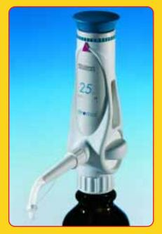
CERAMUS<sup>®</sup> bottle-top dispensers have a unique ceramic piston in a borosilicate glass barrel which guarantees the highest degree of chemical resistance, without abrasion or swelling due to solvent effects. Dispensers fit bottles with A 45 threads and include threaded adapters A 32, A 38, and S 40.
