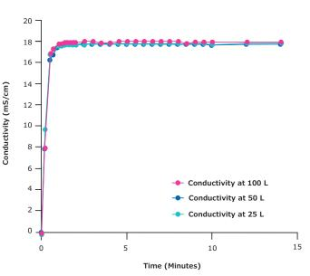
Figure 2. Conductivity vs. Mixing Time at 100 L, 50 L, and 25 L at 400 rpm.
