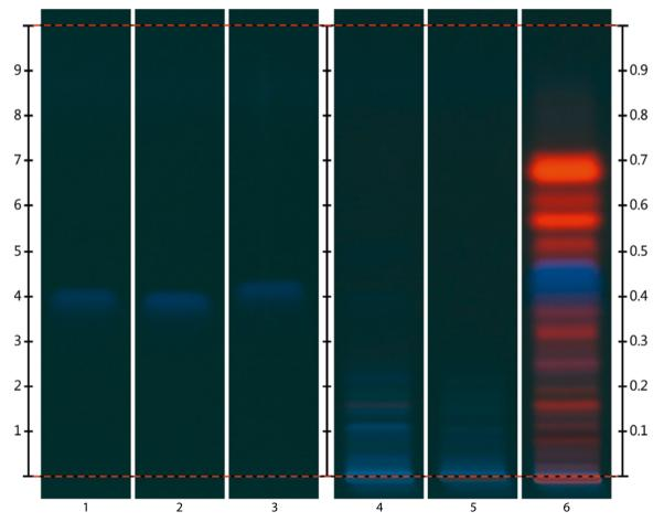
Figure 6. Chromatogram under UV 366 nm. Track 1: Ginkgolic Acid C15:1; Track 2: Ginkgolic Acid C13:0; Track 3: Ginkgolic Acid C15:1; Track 4: G. Biloba Leaf Powdered Extract 05485001; Track 5: G. Biloba Leaf Dry Extract; Track 6: G. Biloba Powdered Leaf
