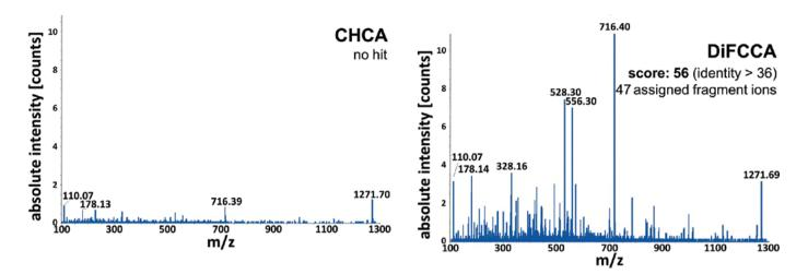
Figure 6. CID-MS/MS Spectra of Protonated Peptide LFTGHPETLEK (m/z 1271.66) Resulting from a Myoglobin Digest (50 fmol). Mass Spectrometer, QStar Pulsar I (MALDI-QqQ-OTOF); Collision Gas, Argon; Collision Energy, 90 eV; Data base, NCBInr; Organism, Other Mammals; Enzyme, Trypsine; Max. No. of Missed Cleavages, 1; Variable Mod., CAM-C and Met.-Ox.; Precursor Tolerance, 25 ppm; MS/MS Tolerance, ±0.1 Da
