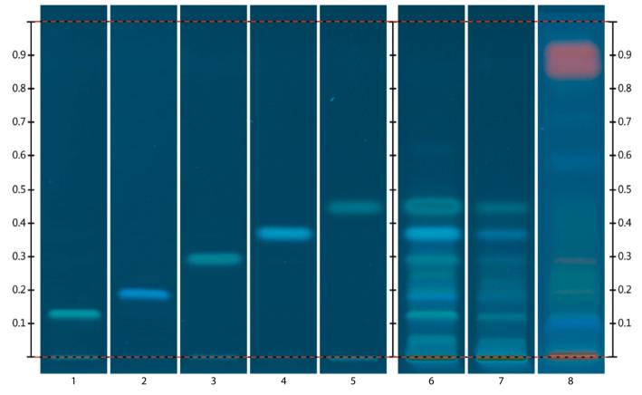
Figure 4. Chromatogram under UV 366 nm after Derivatization. Track 1: Ginkgolide C; Track 2: Ginkgolide J; Track 3: Ginkgolide B; Track 4: Ginkgolide A; Track 5: Bilobalide; Track 6: G. Biloba Leaf Powdered Extract 05485001; Track 7: G. Biloba Leaf Dry Extract; Track 8: G. Biloba Powdered Leaf
