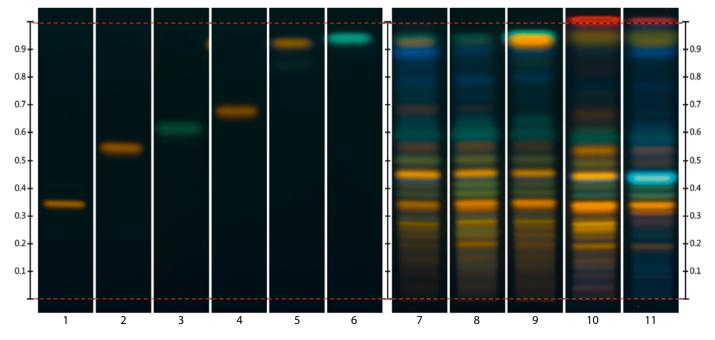
Figure 2. Chromatogram under UV 366 nm after Derivatization. Track 1: Rutin; Track 2: Quercetin-3-glucoside; Track 3: Apigenine-7-O-glucoside; Track 4: Quercitrin; Track 5: Quercetin; Track 6: Kaempferol; Track 7: *G. Biloba* Leaf Powdered Extract 05485001; Track 8: *G. Biloba* Leaf Dry Extract; Track 9: *G. Biloba* Leaf Dry Extract Adulterated with Quercetin; Track 10: *G. Biloba* Powdered Leaf; Track 11: *G. Biloba* Powdered Leaf (Golden Ginkgo)
