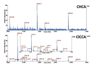
**Figure 3.** MALDI Mass Spectra of a Tryptic In-solution Digest of  $\beta$ -casein (Containing 10%  $\alpha$ -casein) Using CHCA or CICCA as Matrix. m/z Section 2,000–2,500 Da; Shots per Spectrum, 500; Polarity, Positive; Total Sample Load, 50 fmol. For More Information, See Reference 2
