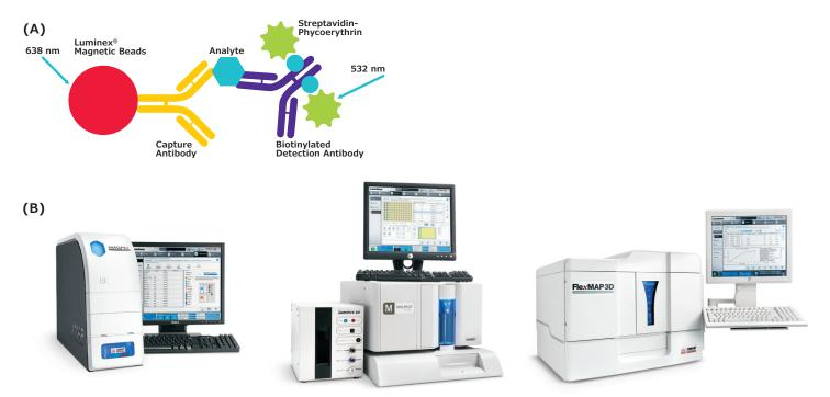
Figure 1. (A) Luminex<sup>®</sup> protein detection immunoassay method. (B) Instruments for use with MILLIPLEX<sup>®</sup> kits (left to right: MAGPIX<sup>®</sup>, Luminex<sup>®</sup> 200<sup>™</sup>, FLEXMAP 3D<sup>®</sup>).
