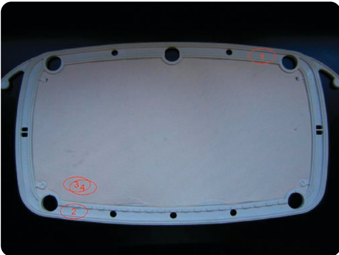
Figure 22. Location of spore strips inside Millistak+® Pod filter.
