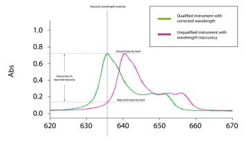
Figure 1. Wavelength Shift Causing an Incorrect Measurement
