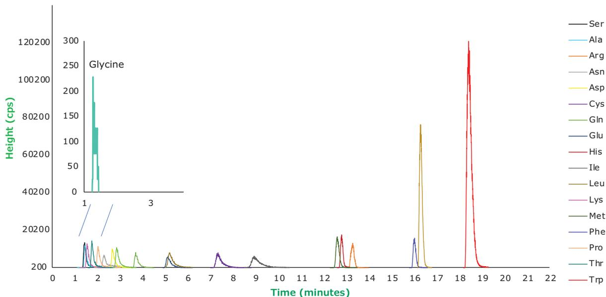
**Figure 2:** Separation of 20 underivatized amino acids by LC-MS/MS. Conditions: Column: Supel™ Carbon LC, 10 cm x 2.1 mm I.D., 2.7 μm; Mobile Phase: [A] Water (0.1% (v/v) DFA); [B] Acetonitrile (0.1% (v/v) DFA); Gradient: Hold at 0% B for 7 min; 0% B to 5% B in 5 min; 5% B to 100% B in 10 min; Flow Rate: 0.2 mL/min; Column temp.: 12 °C; Detector: MSD; Injection: 1.0 μL; Sample: Amino Acid Mix, varied concentration, water (0.1% (v/v) DFA)
