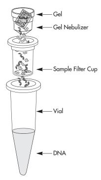
Place gel slice into Gel Nebulizer sample cup assembly and seal device with the cap attached to vial.
