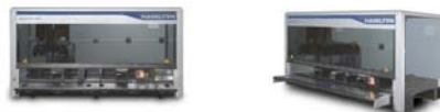
Figure 2. The Hamilton MICROLAB STAR system equipped with 96 head, 8 channel head, iSWAP, shaker and Automated Vacuum System was used for the ADME applications. The Solubility assay uses the 96 head, while the HDM-PAMPA assay uses both the 96 and 8 channel heads. The Total Drug Analysis assay can be done with either the 96 head or the 8 channel head.
