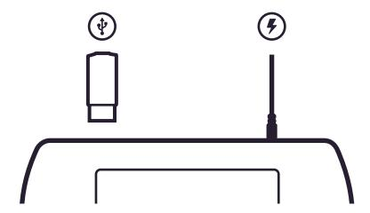
Insert a USB drive into the Data Port on the back of the Control Unit, next to the power connector.
