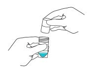
11. Place the cap onto the External solution container. Place the External solution container vertically inside the constant temperature box. Set the constant temperature box to 30 °C.
