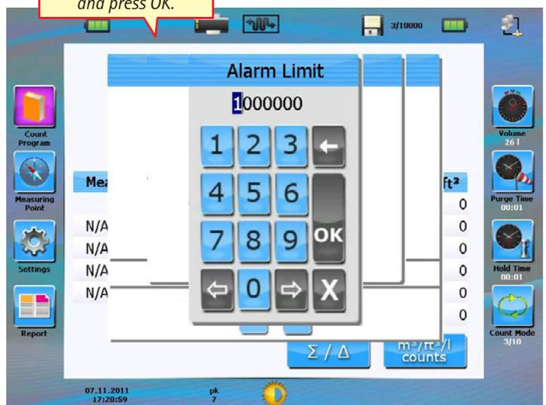
Change the particle size of channels by using the arrows or press the figures to access the numeric pad using the key pad enter the size you require and press OK.
