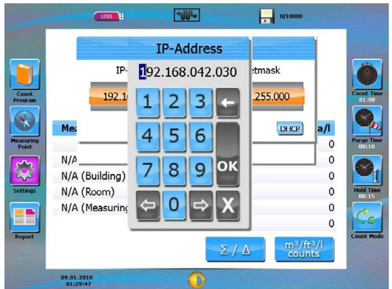
Type in the required IP Address. Then press OK.
