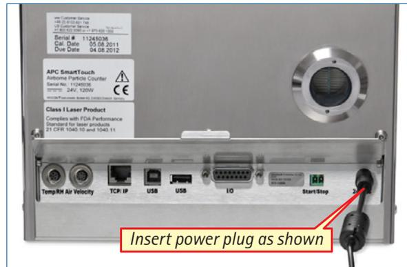
After this initial 4 hour charge the instrument can either be used via the external power supply or the internal rechargeable lithium ion batteries.
