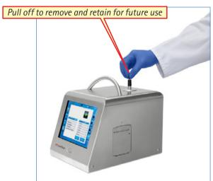
Now fit the correct isokinetic probe by pushing down.
