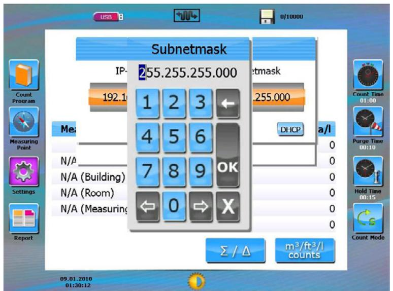
Type in the required IP Address and then press OK.
