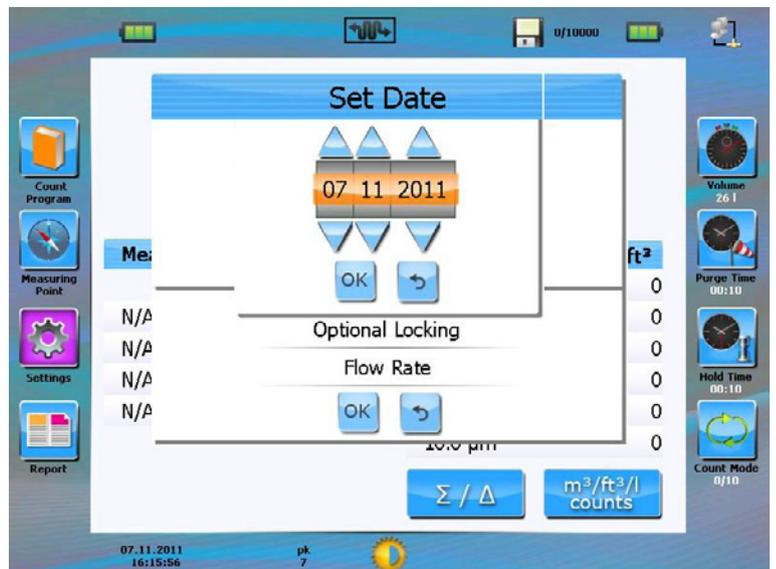
The buttons above and below are used to increase or decrease the date. When correct press OK.
