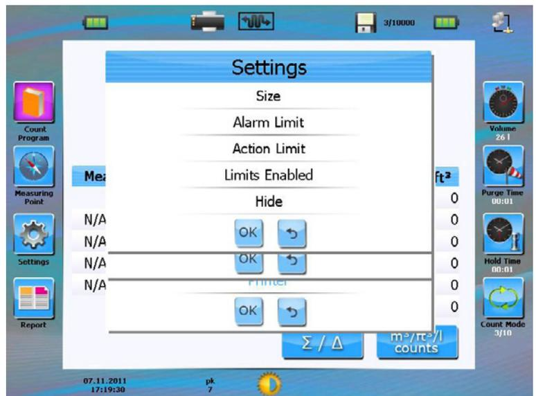
In this screen you can set the alarm limit to a desired level of particles. An alarm (audible and visible, the channel that generated the alarm will be highlighted in orange) will occur when the level has been passed.
