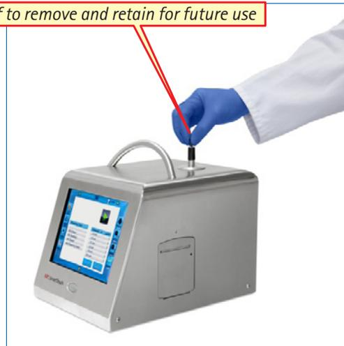
Now fit the correct isokinetic probe by pushing down.
