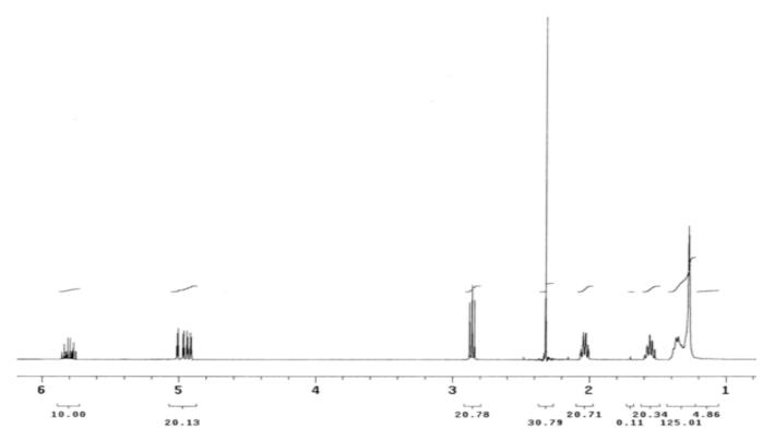
Figures 3 and 4 show the H<sup>1</sup>-NMR of the thioacetate (1) and the resulting free thiol (2) respectively. This free thiol can be directly used to create self-assembled monolayers.
