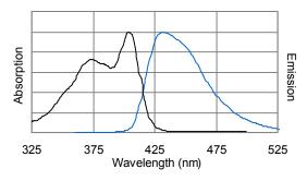
$\lambda_{abs}$  = 404 nm (PBS buffer, pH 7.4)  $\lambda_{em}$  = 431 nm (PBS buffer, pH 7.4)
