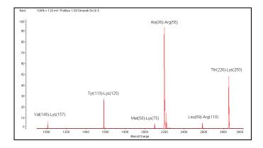
The substrate protein, carbonic anhydrase II (0.5  $\mu$ g), was separated on a 4–20% Tris-Glycine gel. The spot was removed and digested using the protocol for in-gel digestion. The matrix ( $\alpha$ -cyano-4-hydroxycinnamic acid) was prepared at 10 mg/ml in 70% acetonitrile with 0.1% TFA. The digest solution was desalted using a C<sub>18</sub> ZipTip and 1.5  $\mu$ l of the matrix solution was used to directly elute the peptides onto the MALDI target.
