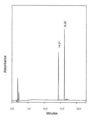
Insulin B chain, oxidized (100  $\mu$ g) was digested with 2  $\mu$ g of trypsin for 18 hours at 37 °C in 100  $\mu$ l of 100 mM Tris-HCl, pH 8.5. A 10  $\mu$ g aliquot was separated on a Supelco Discovery<sup>®</sup> C<sub>18</sub> column (15 cm × 4.6 mm, 5 micron, Catalog Number 504955), using a 20 minute linear gradient from 5-50% B at 1 ml/min with UV detection at 214 nm and by mass spectrometry. Solvent A: 0.1% (v/v) TFA in water and Solvent B: 0.08% (v/v) TFA in acetonitrile.
