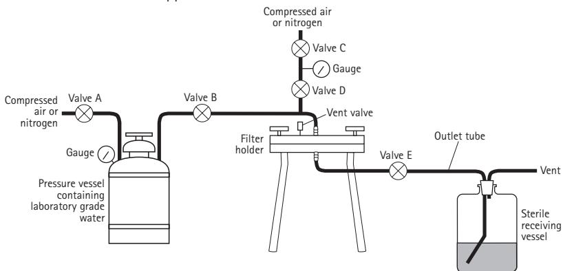
**NOTE:** Filter holder outlet tube or receiving vessel must have a clear portion in order to determine when the bubble point has been reached.
