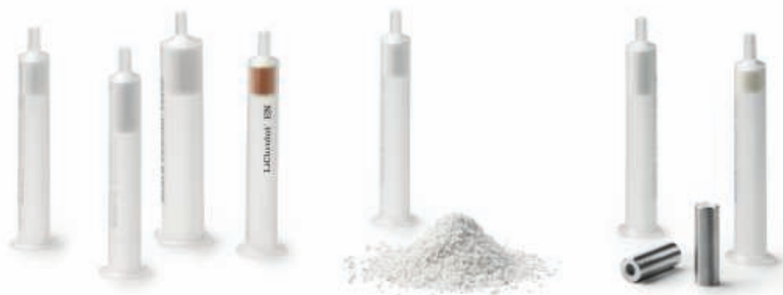
Figure 2 Various LiChrolut® cartridges suitable for the sample preparation of samples with high salt and matrix load. The type of stationary phase (e.g., reversed phase, cyano) can be chosen according to the specific needs of each sample.
