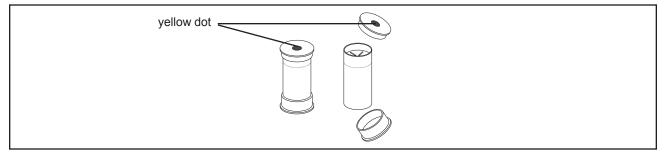
Push the plug fully into the tapered end of the spin column using the insertion tool.
