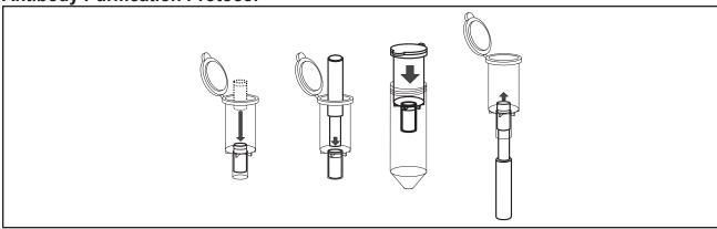
After loading the plug into the spin column and placing the spin column into a centrifuge tube, follow the procedure below.
