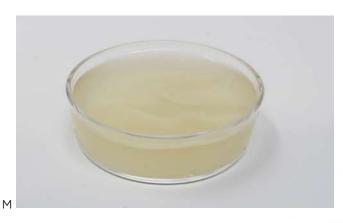
13. The bath should be as bubble-free as possible (N). Tapping firmly against the table can force large bubbles to the surface. The bath should not move easily if the container is tilted (O). Be gentle when tapping glass dishes.
