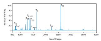
Figure 3. The sample was desalted using a ZipTip™ C18 pipette tip from Millipore and eluted directly onto the MALDI target using the MALDI matrix (α-cyano-4-hydroxycinnamic acid, 10 mg/ml in 70% ACN, 0.03% TFA). MALDI analysis was performed in the reflection positive ion mode.
