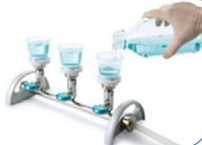
4. Open the valves and start the filtration. To ensure an optimal retention, apply a vacuum of 0.6 to 0.8bar.
