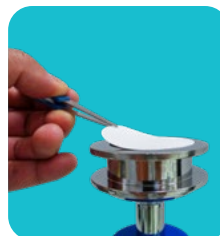
Placing filter on manifold head
