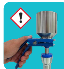
Installing filter funnel on manifold
