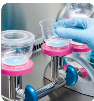
EZ-Fit® Filtration Unit set-up
