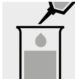
Pipettare 0,50 ml di SO<sub>4</sub>-1 in una provetta.
