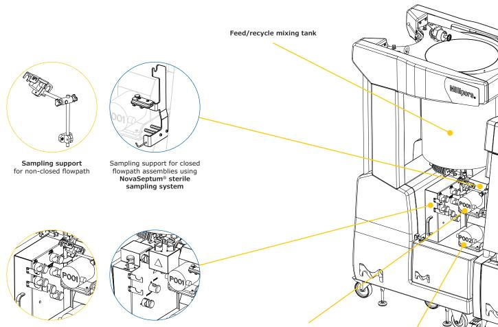
Pump cart and transfer manifold controlling 5 inlets on transfer line
