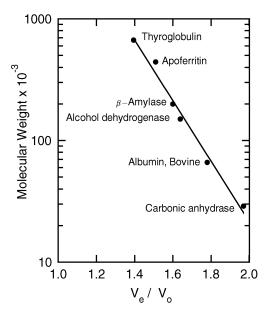
5. Elution Volume (V<sub>e</sub>) Determination for an Unknown Protein – Apply the unknown sample to the column at an appropriate concentration using the same sample volume, fraction size, and flow rate as used for the blue dextran and the protein standards. Determine the V<sub>e</sub> of the unknown using the same methods applied to the standards. Calculate the V<sub>e</sub>/V<sub>o</sub> for the unknown and determine its molecular mass from the standard curve.
