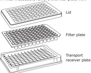
the receiver plate to retrieve the permeant.
