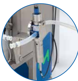
Pre-column instrumentation for conductivity and pH measurement
