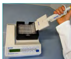
7. Washing (Removal of unbound components, 2x 1 min)
