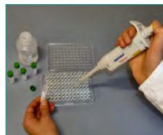
3. HybriScan® - test solution (Forming of "sandwich complexes" between specific probes and the sample, 10 min)
