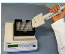
5. Immobilisation (Binding of the "sandwiches" to the binding plate, 10 min)
