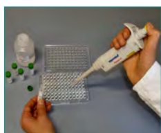
4. HybriScan® test solution (Forming of "sandwich complexes" between specific probes on the sample, 10 min)
