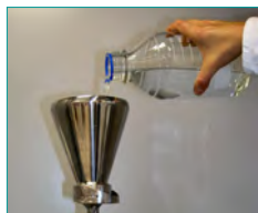
1. Sample filtration (250 – 1000 ml water, 15 min)
