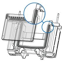
For buffer dams (BDAM1), the notched side of the gasket must face the buffer dam to form a proper seal.
