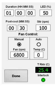
To change the set point of a given parameter select it on the touch screen. This will provide a display corresponding to the parameter you have chosen as shown on the right. The dial may be rotated to select the desired setting. Alternatively, pressing the "KEY" button will allow the user to enter an exact value. Pressing the "DONE" button will accept the value.
