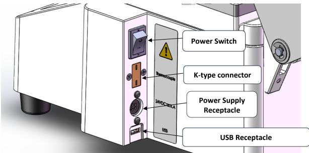
The unit must be powered with the supplied power supply (85-264V, 50/60 Hz, Full Range).
