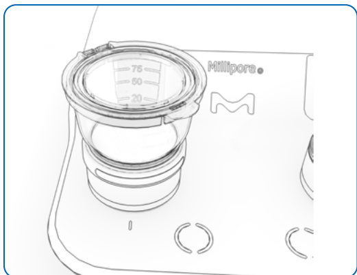
Figure 16: filtration unit placement
