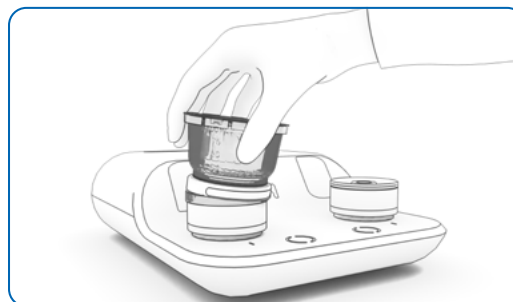
Figure 19: Filtration unit tilted for removal
