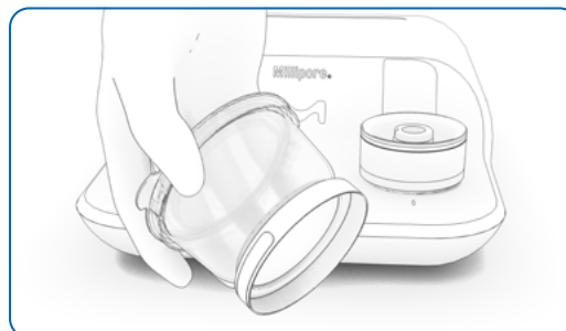
Figure 20: checking of the membrane convex shape
