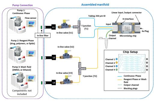
**Figure 1:** Schematic of the microfluidics setup for the Dolomite Microfluidics system. The manifold is supplied preassembled. The microfluidics chip is packaged separately. In-line filters are supplied for connection to microfluidic pumps. More information can be found in the corresponding NanoFabTx™ Microfluidic - nano Device kit (Cat. No. 911593).
