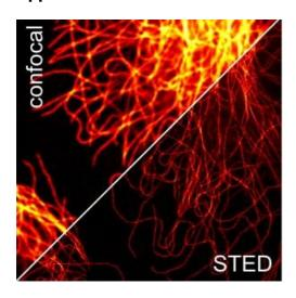
Comparison of a confocal (upper half) and the corresponding STED (lower half) microscopy image obtained with an Abberior STAR 635 labeling.
