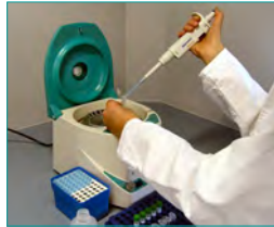
2. Zellyse (2 ml Probe, 13.000 rpm; 37°C, 45-60 min)
